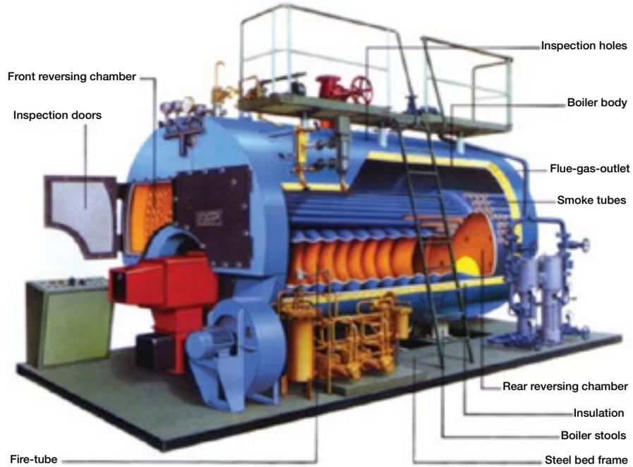
Figure 3.2 - Typical fire-tube boiler
