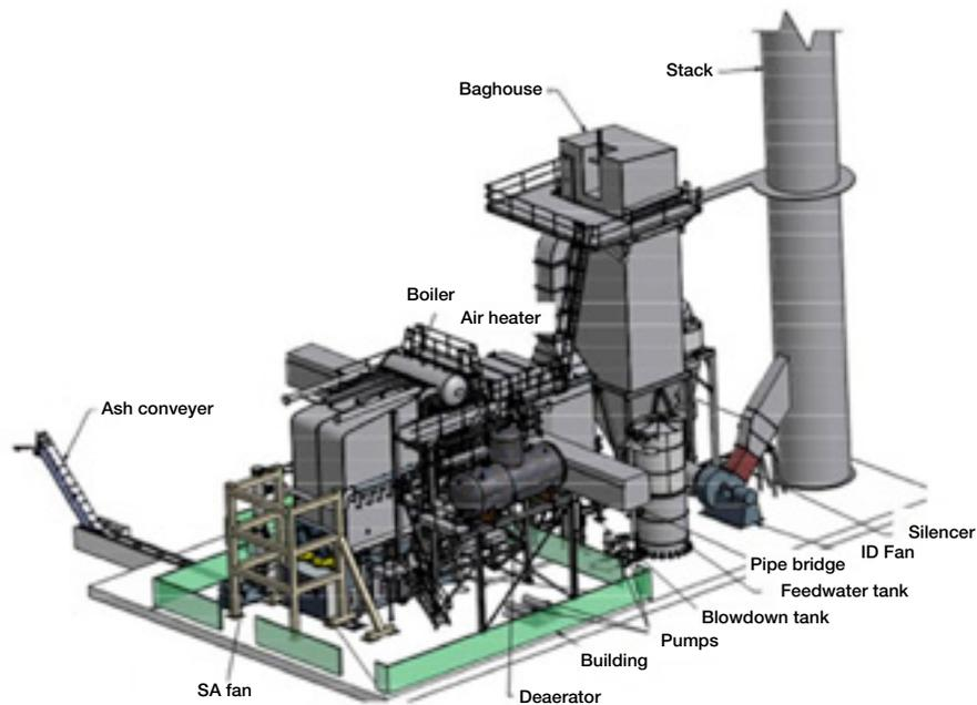
Figure 3.3 Typical large industrial coal fired boiler
