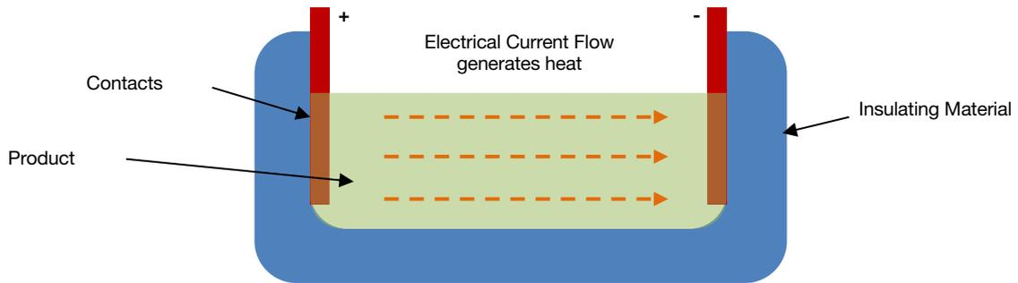
**Figure 1. Direct resistance heating of liquids**
