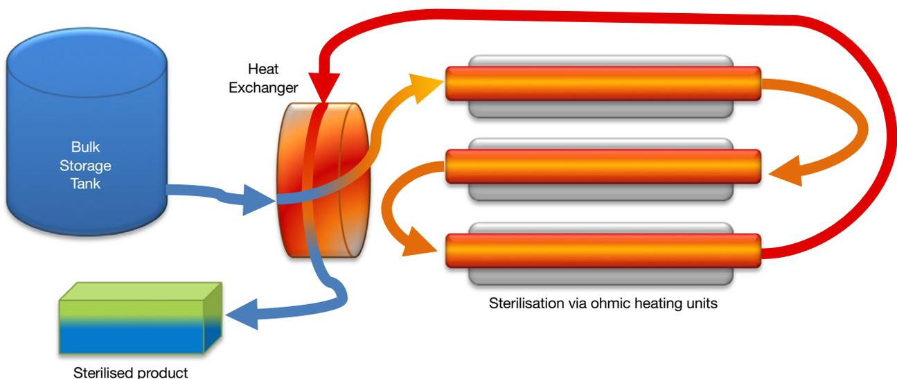
Figure 7. Pasteurisation and sterilisation using Ohmic heating with a heat exchanger
