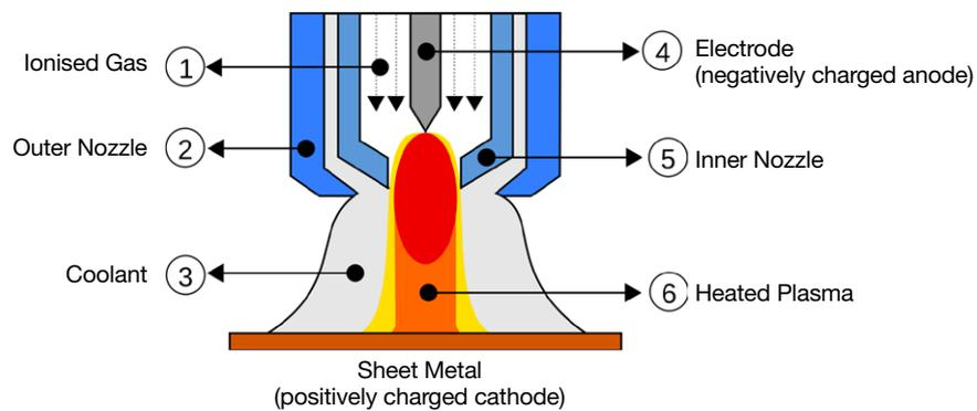
**Figure 8. Basic plasma cutter operation**
