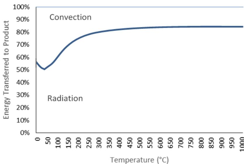
Figure 3. Convection and Radiation heat transfer relative to temperature
