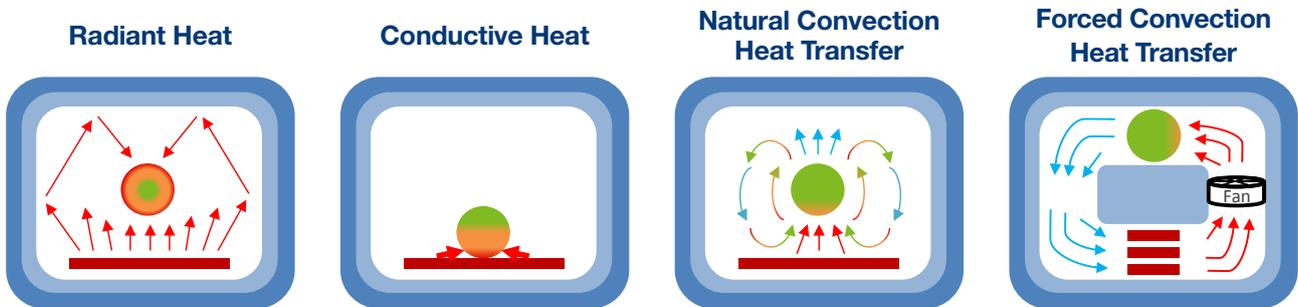
Figure 2. Conductive, Radiative and Convective heat transfer
