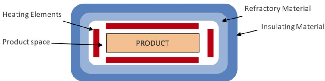
Figure 1. Elements and insulation in relation to product
