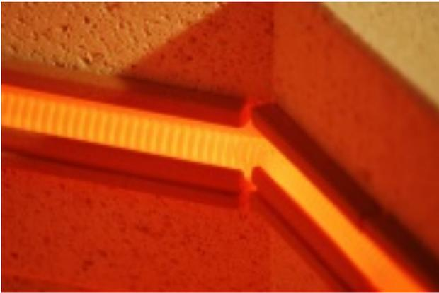
**Figure 4. Spiral elements embedded in kiln insulation**
