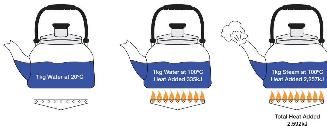
Figure 8: Steam Generation at Atmospheric Pressure
