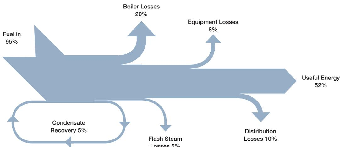
Figure 3: Steam System Energy Balance “Average” System Efficiency
