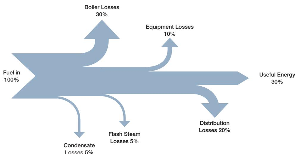
Figure 2: Steam System Energy Balance "Poor" System Efficiency
