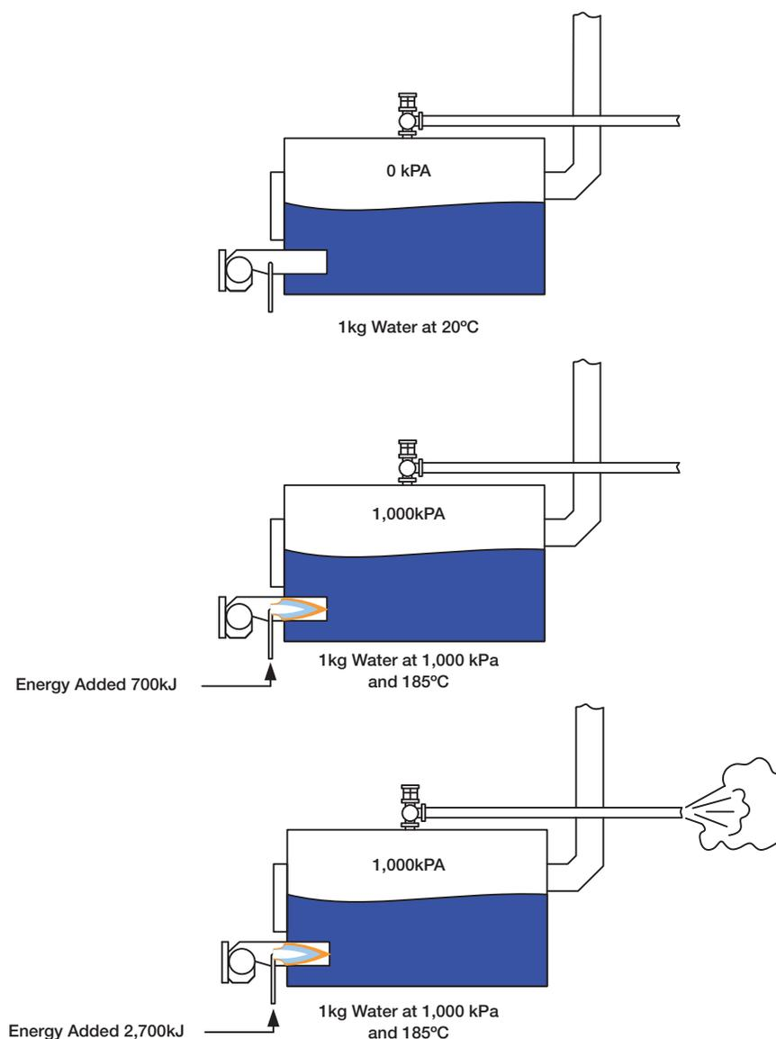
Figure 9: Steam Generation under Pressure
