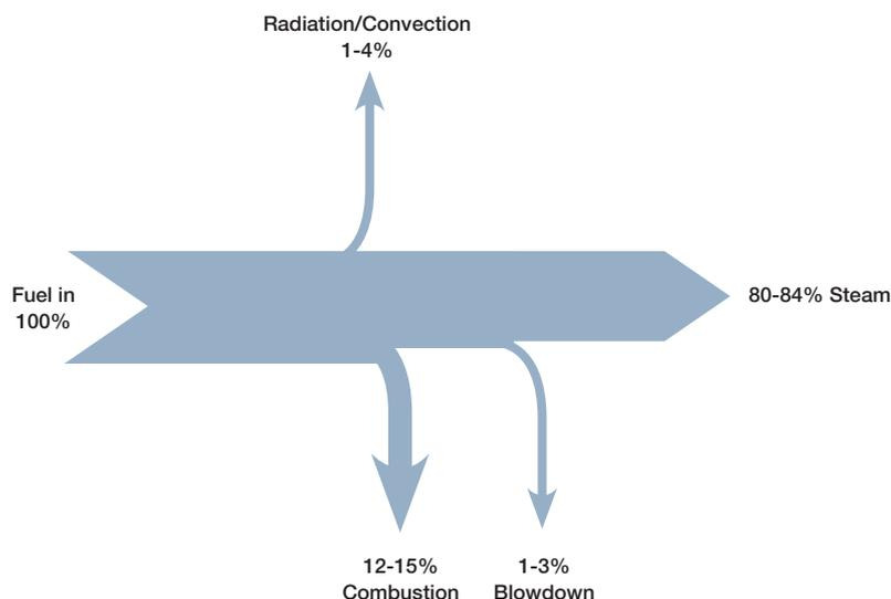
Figure 7: Typical Boiler Energy Losses
