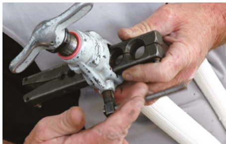
Figure 6.18 Flare the end of the tube (B)
