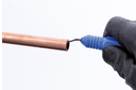
Figure 6.2 Step 1: Cleaning the tube end
